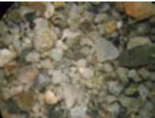
fig. 10. Sand grains of the mortar under the microscope
