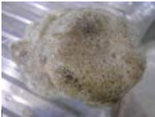
fig. 9. HCl (hydrochloric acid) test to determine presence of calcium carbonate
